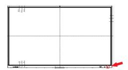
**Power button** Press once for standby mode. Press and hold to turn display off.
